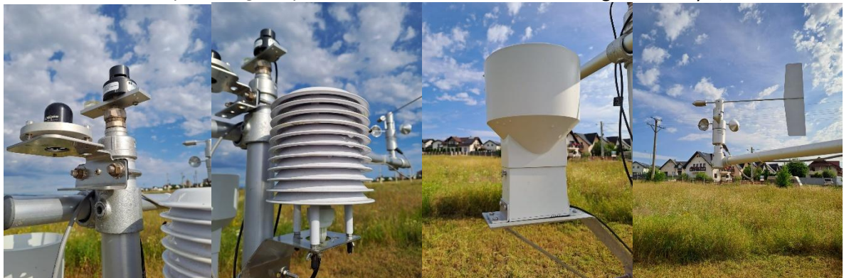
Components from left to right: radiation sensors, mini weather shelter with temperature and humidity sensors, rain gauge, anemometer, and wind vane
